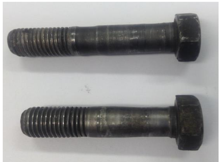
Photo 3: Bolts that were holding a loose alternator. The give away was that the alternator belt was loose.
