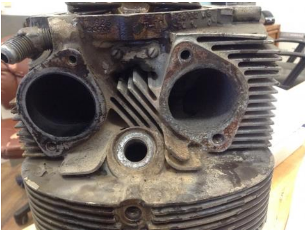
Photo 1: Eroded exhaust boss. Hint, it is the one on the right
