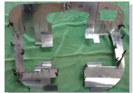
Photo 6: Baffle assembled with Clecos. This should readily slip onto an O-320 saving many hours of cut and try.
