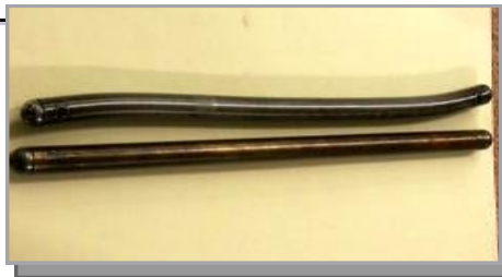
Photo 3: Push rod from the damaged cylinder along side a good pushrod
