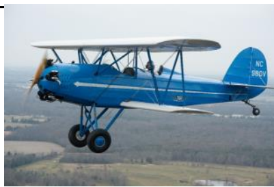
Model "BK" powered by the Kinner K-5; https://airandspace.si.edu/multimedia-gallery/6612hjpp
