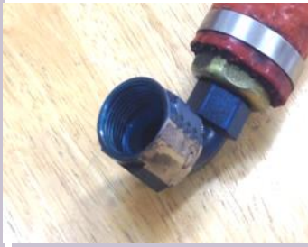
Photo 7: Oil hose worn by chafing
