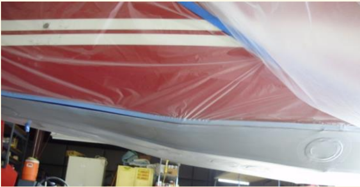
The Belly Getting Silver Dope. Note the use of Fine Line Tape before applying the blue masking tape.
