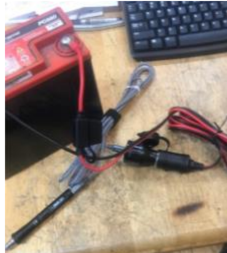
Photo 3: Smart soldering iron portable rig.
