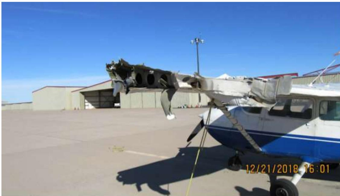
The NTSB has released its factual report on a 2018 incident that ended with the pilot of a Cessna 172 coaxing the aircraft ten miles to a safe landing missing four feet of the left wing and most of the trailing edge. The pilot was uninjured. The aircraft was on a pipeline patrol south of Abilene, Texas on Dec. 21, 2018 when it hit a tower guy wire. The pilot was able to maintain control of the plane and land at Abilene.
