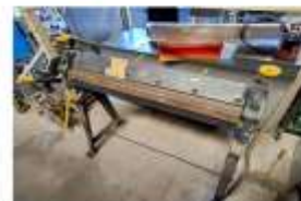
Peck Stow + Wilcox Sheetmetal Brake
