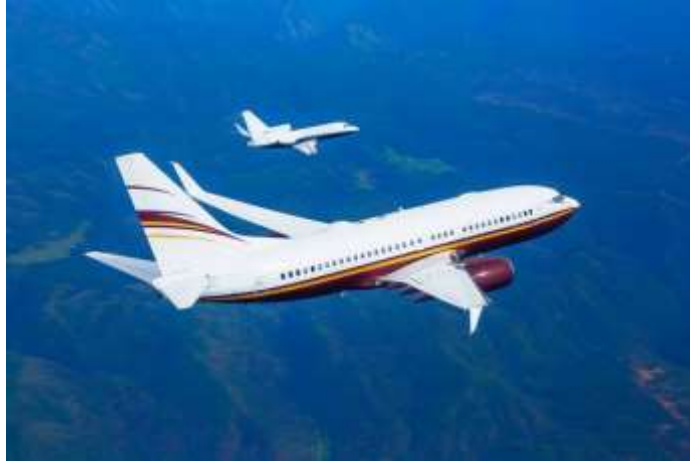
A Blended Winglet-equipped Falcon 50 and Split Scimitar Winglet-equipped BBJ in flight. Aviation Partners, Inc.
