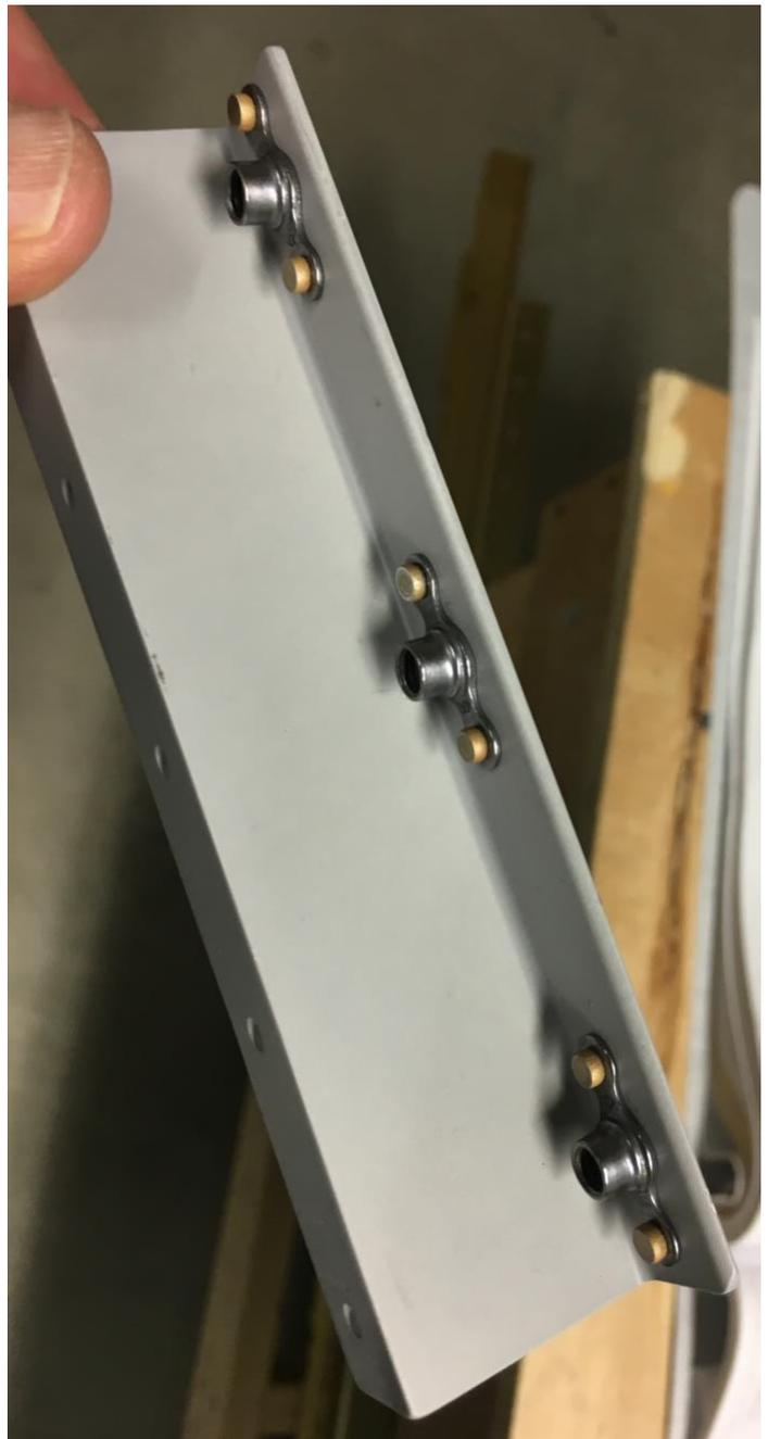
A z-bracket with nutplates installed.
