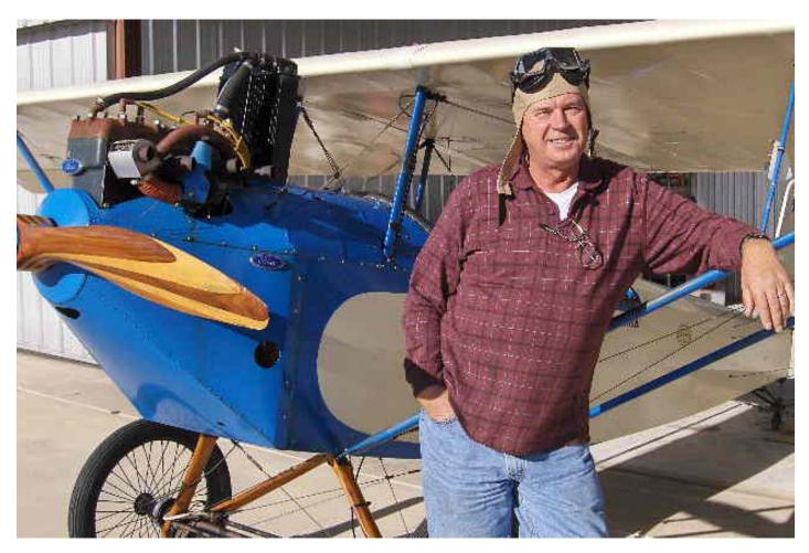
Note the powerplant: the engine from a Ford Model A car! The black object just forward of the wing is the radiator. This pulls the "Piet" along at 63 mph, according to Ron. By way of contrast, the Pietenpol's hangar mate is a Glasair, also owned by Ron. It cruises at 200 knots, which is nearly four times as fast. But it also has a 300 hp engine, compared to the 40-something produced by the Model A engine.
