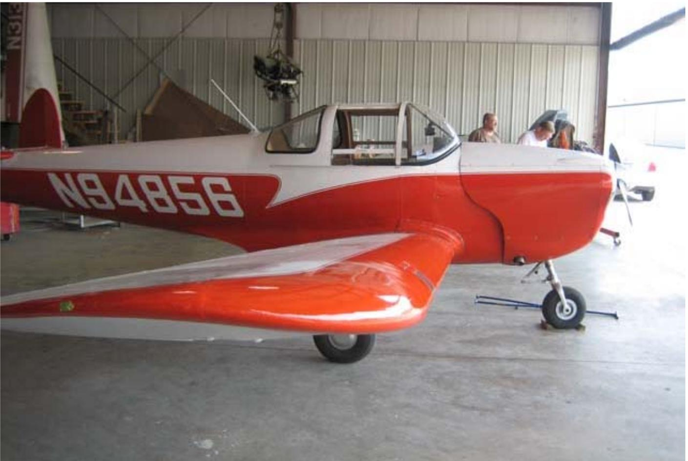
Start up is a bit interesting. One pump of the primer, turn the key to "both" magnetos, and then PULL the starter handle out, hard. This engages the starter, and the little 85 horsepower Continental pops right over. The pull starter seems odd but remember that contemporary aircraft of the Ercoupe -- Taylorcrafts, Luscombes, Cessna 120s -- all had to be hand-propped, so this set up was way ahead of its time.
