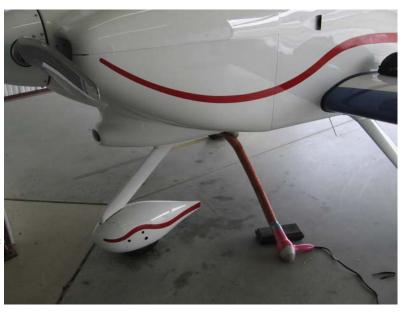
engine when it is very cold is due to the unique thermodynamic qualities of interacting aluminum parts with steel parts. They have different rates of expansion and contraction and it is possible for the aluminum crankcase and crankshaft bearings to actually lock up on the steel crankshaft in sub zero weather. If you start an engine at that time it isn't good for anybody! I decided that a little pre heating was in order.
