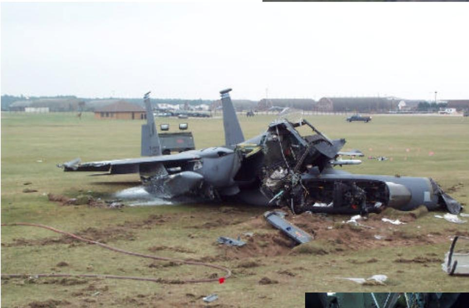
way, the front end dug into the ground causing the jet to stand up on its nose. At that point, the fuselage broke apart just forward of the intakes and aft of the rear cockpit and then bent around and underneath the left side of the aircraft.
