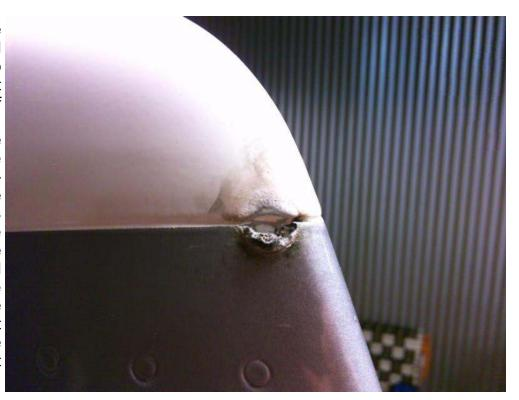
Anyway, the irony of the situation has not escaped me. Struck by lightning, on the 4th of July, right next to the lightning bolt graphic I put on the tail. Moral of the story: don't tempt fate by putting a lightning bolt on the tail of your airplane, and then leaving it outside in a thunderstorm. :)
