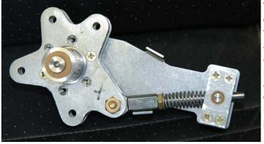
We went through at least 11 iterations of the design – refining it each time. The original factory system does not use bearings for the aluminum push rods, and it does not take into account the arc that results from the movement of the bell crank. This results in friction and binding. One has to use enough force to overcome this friction and then push the door handle through over center and then continue pushing to close the door. Our system takes
