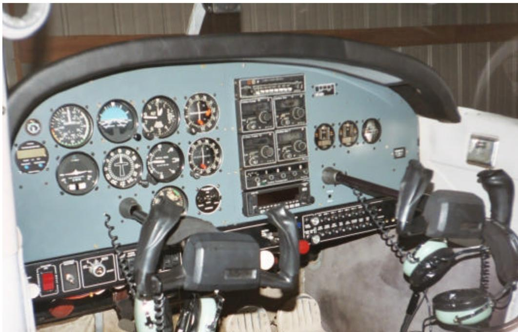
which made a standard center radio stack possible. Along with the STC, Avion custom builds a nice "standard six" instrument panel for any model. They paint and silk-screen the finished product for a nice look too.
