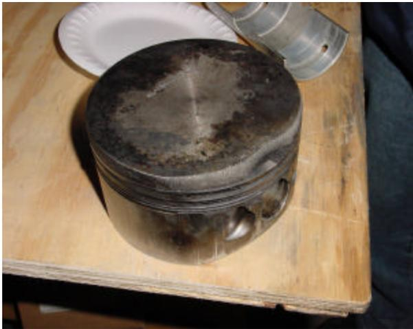
from his LongEze's O-290 that developed ringed wear patterns in the side wall. Ron brought a disassembled master solenoid that had recently failed after a mere 2000 or so hours on his LongEze. The overall message is, if you are working on your engine or want to learn about such things, we have a wealth of knowledge in the chapter. Be sure to come to our meetings and take advantage of this and share your knowledge with the rest of us. John also showed us his latest project,
