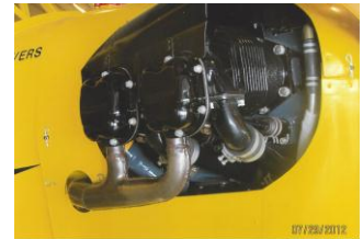
Yes . . . that is Continental Gray and the engine has Champion C-26 spark plugs.
