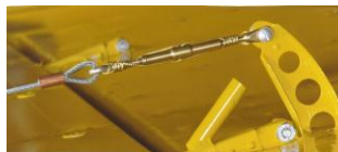
Note the Piper ‘single squeeze’ on the cable. Brass safety wire was common in 1946.
