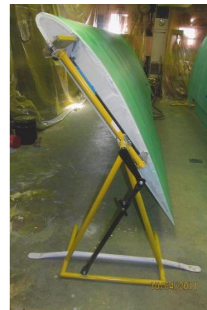
A fixture was developed to permit Marv to rotate the wing by
