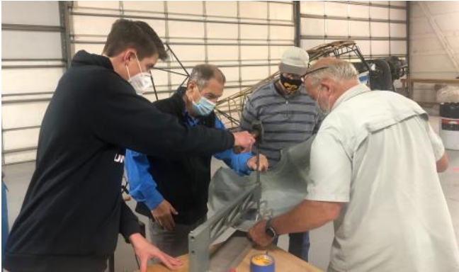
Bridger using Lyle's C-frame to set a rivet in cowling door.
