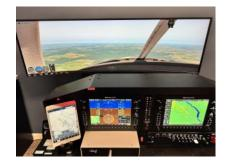
The BATD is certified under F.A.R. Part 61 and F.A.R. Part 141 requirements. It is currently configured for Piper Archer and Cessna 172 aircraft with dual G1000 flight displays.
