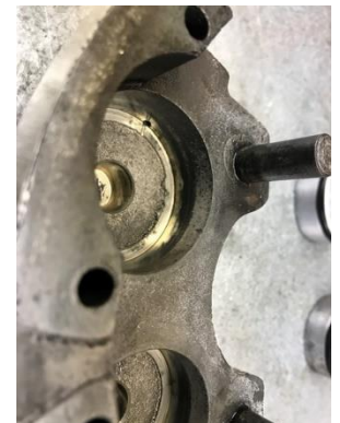
Moisture in the brake system can cause corrosion and leaks from the caliper pistons. Photo courtesy of Jeff Simon.
