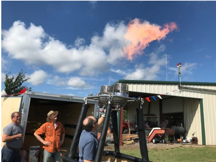
This is the main burner that fills the Balloon!
