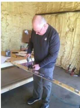
Frank showing onlookers how to use Cleco pins!
