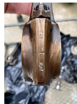
All 4 Rods were ground on for weight redistribution.
