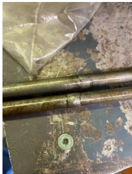
6 of 8 pushrods had been welded together!
