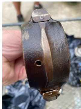
All 4 Rods were ground on for weight redistribution.
