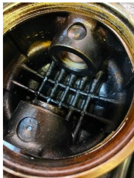
3 of 4 Pistons were drilled into for weight balancing.
