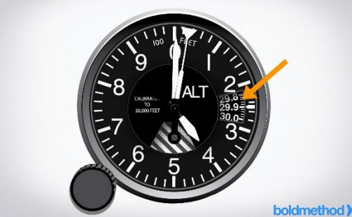
Kollsman Window On Traditional Altimeter
