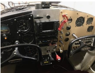
“Roughing” out instruments panel for testing. Powder coating when new panel is finalized and cut.
