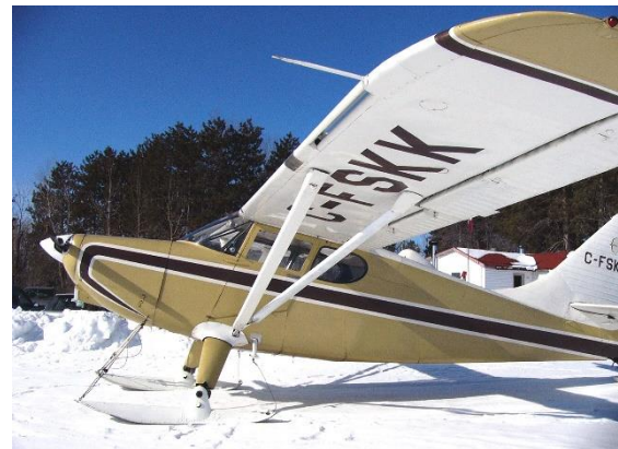
A Canadian 1949 model Stinson 108-3 on skis. The partial span leading edge slot is visible.
