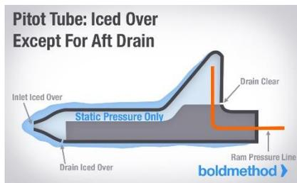
If this happens, all of your ram air will leak out the drain, and you're left with nothing but static pressure. And if that happens, your airspeed goes to 0.
