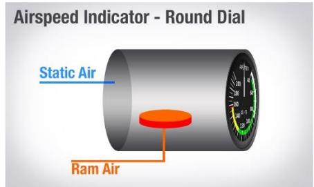
It does this by filling up the case of the instrument with static air, and filling something called an "pressure diaphragm" (the orange thing in the diagram above) with ram air. There are also some gears involved to make your airspeed needle move, but to keep things simple, as the diaphragm fills up with more ram pressure, it expands, and your airspeed goes up.
