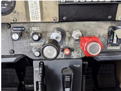
Alcohol-based disinfectant produced by a distillery and sprayed on an Atlas Aviation Skyhawk's instrument panel damaged the panel near the power quadrant. Photo courtesy of Deric Dymerski.
