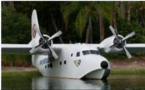
Grumman HU-16 Albatross is a large, twin-radial engined amphibious seaplane
