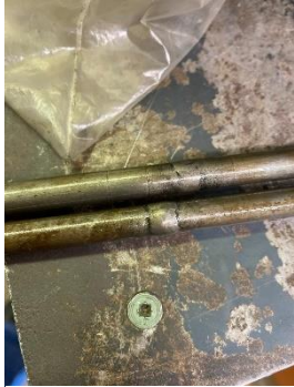
6 of 8 pushrods had been welded together!
