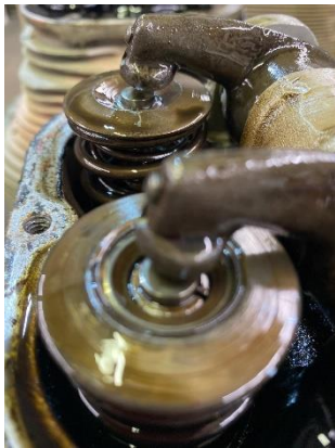
Damage caused to valves and springs due to not having the proper lengths!
