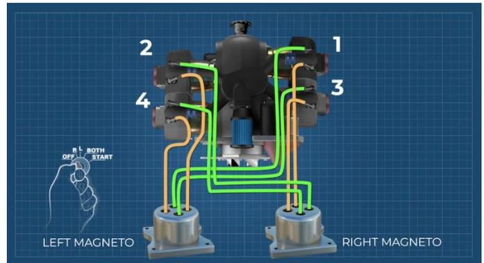
The purpose of the magneto is to generate a high voltage pulse of up to 20,000 volts, sufficient to create the spark required by the spark plugs to ignite the fuel inside a piston.
