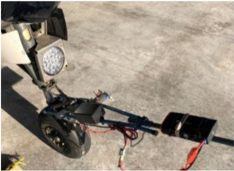
Franken-tow hooked up to Adam's Debonair ready to pull the aircraft both in and out of his hangar!
