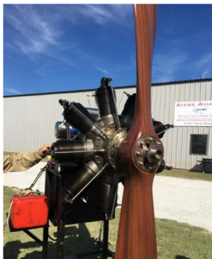
Gnome Engine WWI vintage Sopwith Camel powerplant.
