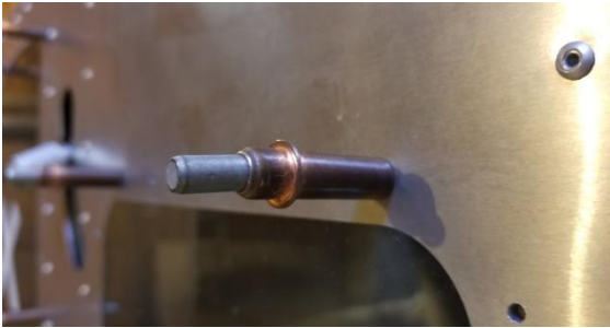
A Cleco fastener (installed on the outside of the Airplane) holding the outer Aluminum and window together.
