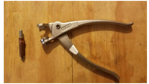
Cleco pliers and a Cleco Fastener
