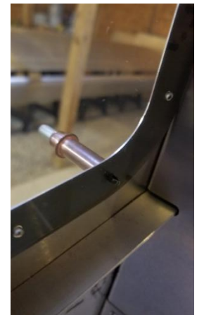
Blind side look of Cleco Fastener holding Window and Aluminum together
