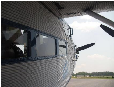
Externally mounted control wires of a Ford Trimotor
