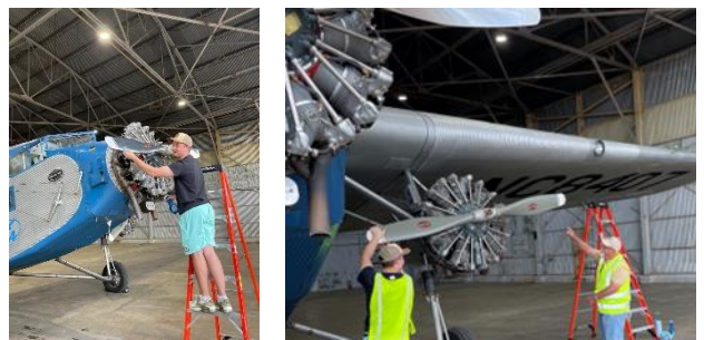
Pulling the engine through and cleaning bugs! Under the supervision of Rick Simmons!
