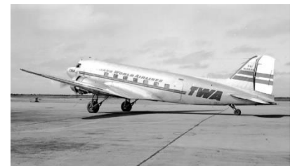
TWA DC-3, a tail wheel (conventional gear) airplane. The rudder and rudder trim are very obvious in this photo.
