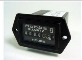
Typical Hobbs meter's: above is a digital unit and below a mechanical.
