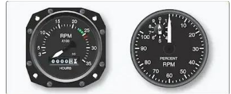
Figure 1. A tachometer for a reciprocating engine is calibrated in rpm. A tachometer for a turbine engine is calculated in percent of rpm.
