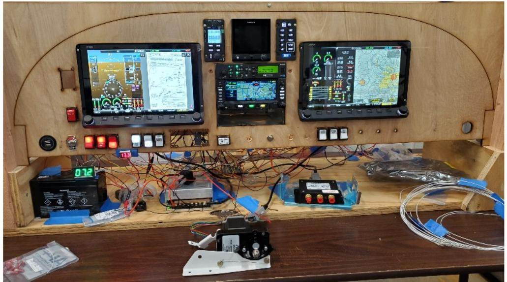
The first picture shows the bench build about as far as we will take it as a prototype. The autopilot servo in the picture had just finished testing. The G5, transponder, and Artex ELT have been flying in the plane so no need to test them on the bench.
