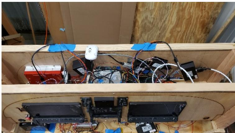
So I highly recommend a bench build and prototyping, both electrical and physical, as much as possible before cutting any aluminum. We’ve already made three fiberboard test cutouts to tweak the placement of switches and controls, and to see how it fits in the airplane. One problem was the first panel design didn’t clear the front vents and had to be made 1/4 inch shorter. This is a whole lot easier to fix in a CAD drawing than with a sheet of aluminum already cut and bent.
