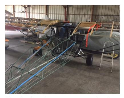
Since the photo the struts were removed, ends welded, reattached, gear removed, leveled and wings adjusted for washout and dihedral.
