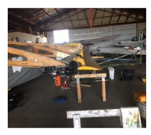
Here is a shot of left wing flaperon in position and ready to be joined up with it's controls. The right side is in correct position to be joined up and holes drilled for second bolts in ribs. We are hoping to start covering next month.
