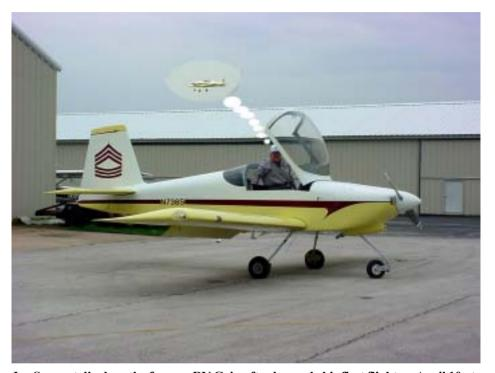
Joe Sargent displays the famous RV Grin after he made his first flight on April 10 at 10:11 am from runway 36 at Smartt Field. All manuevers he tried were easy; stalls straight ahead and no roll trim needed in cruise. 150 mph indicated in the pattern (yeah those puppies are fast) before reducing power. The flight lasted 22 minutes with no squawks, leaks, etc. Joe made a good landing despite his face being stretched all out of shape by his huge smile.
