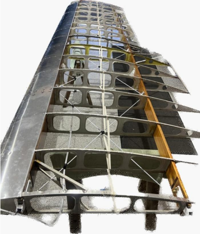
*Figure 2 Complete RH Wing Ready for Covering*
