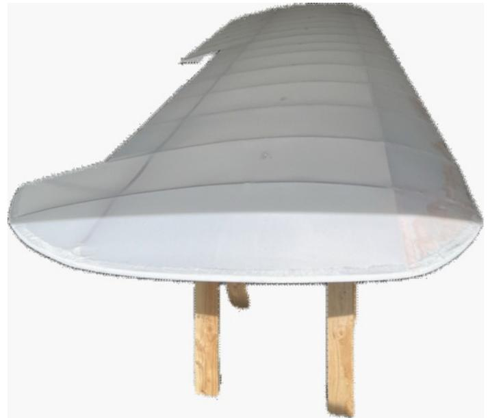
*Figure 3 Covered RH Wing Ready for Poly-Brush*
