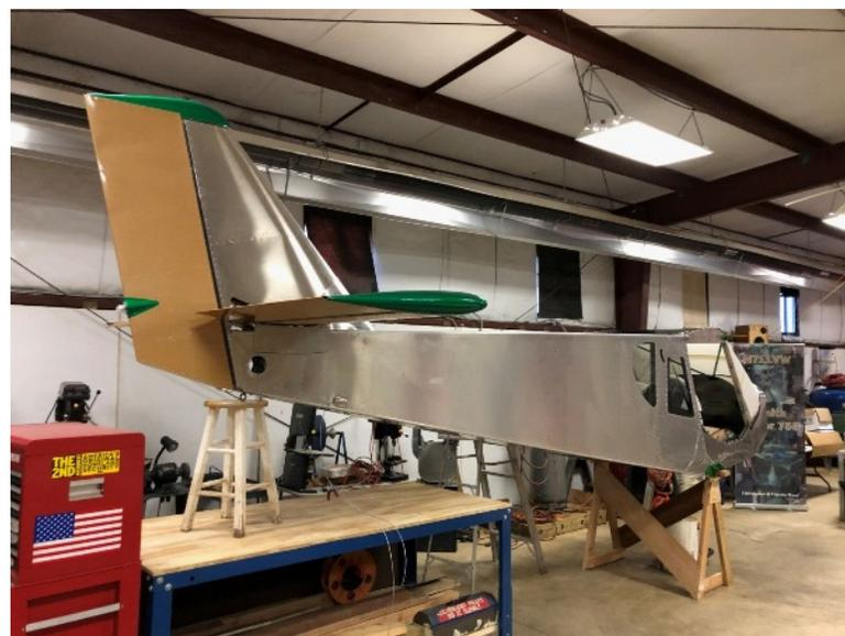
After measuring the length needed for the first wrap of skin down the fuselage side they cut the first piece off a 60 inch wide roll and stretched it out on the aluminum as they began using squeegees to smooth out wrinkles and air pockets beneath the material.
