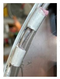
I've learned small things can make a big difference. The two canopy halves are held on primarily with four piano hinges. The two hinges joining the top and bottom halves are fairly straight down the cowling sides. However, the two hinges joining the upper cowling to the curved fuselage have to bend almost 90 degrees. Boy, I was really having to push and
