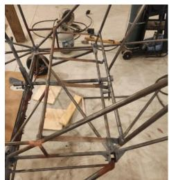
I got to work making a new horizontal seat bar and then made a vertical tube coming down to support the down pressure of the occupant(s). Then I needed to figure out how to hold the wooden seat. I bent up some 1-inch strips on 1/8 inch 4130 plate into "L" brackets and welded them on the back seat tube. This allowed me to drop the seat pan even lower as I needed the headroom beneath the top longeron. I then welded in tabs on the front seat support horizontal.
