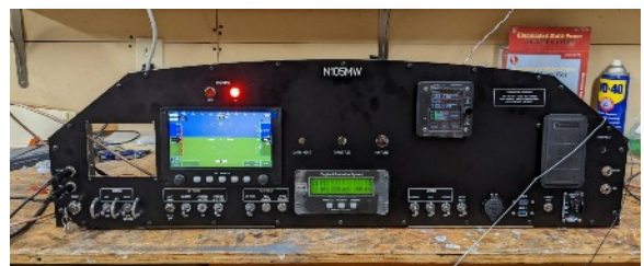
Instrument panel assembled and tested on the bench
