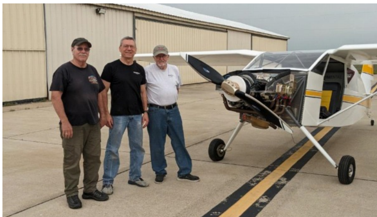
Fuel flow and first engine run complete with the help of Pat Devine and Jim Johnson
