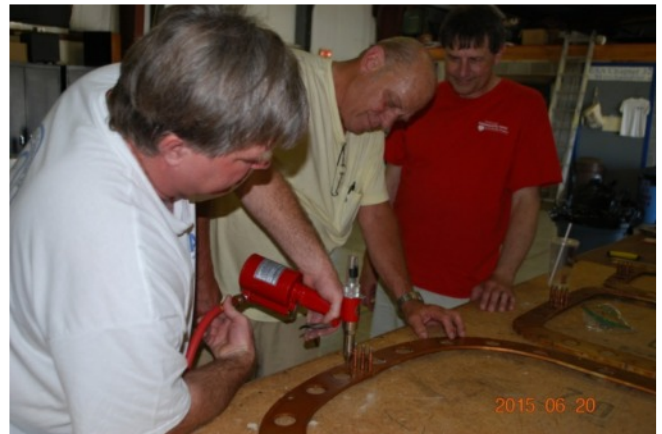
First, the parts are clecoed together.
