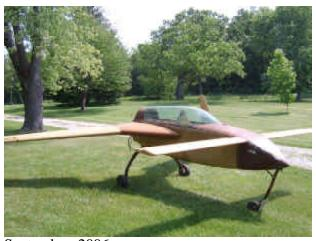
The engine is a Continental c-90, with new bearings, rings, reworked 0-200 cylinders, gaskets, starter, and generator. It needs magnetos and final assembly by either the buyer or a certified tech. The plane has a Long Eze landing gear, airbrakes, electric aileron trim, manual elevator trim, and engine cowling. All controls are installed. If you have any further questions please contact me at 618-488-7471 (Sorento. IL).
