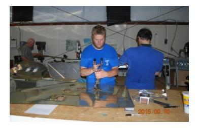
member Chuck started that process out by installing nutplates onto the sheet metal. Then we turned the fuselage section upside down and started elecoing the skin to the frame.
