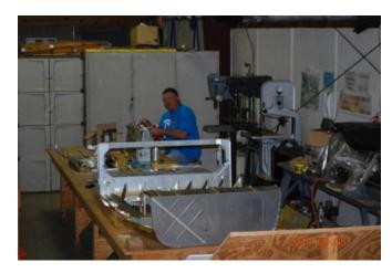
the fuselage structure. We all are amazed at how the fit and quality of the prepunched sheet metal parts are. For the most part, one simply cleco's the parts together and
