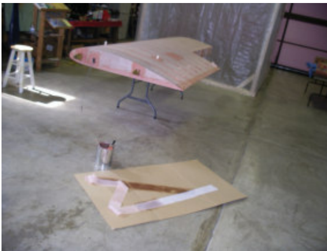
Four inch finishing tape for the right wing before final ironing
