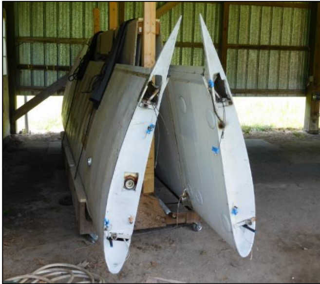
The inside of the wings were dirty and full of both live and dead wasp nests. Fortunately, there was no corrosion and the wood spars were in excellent condition.
