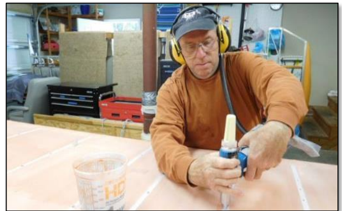
I was very happy to learn that the design of my wings employed rivets, rather than rib stitching, to secure the fabric to the ribs. Rib stitching is a very tedious process.
