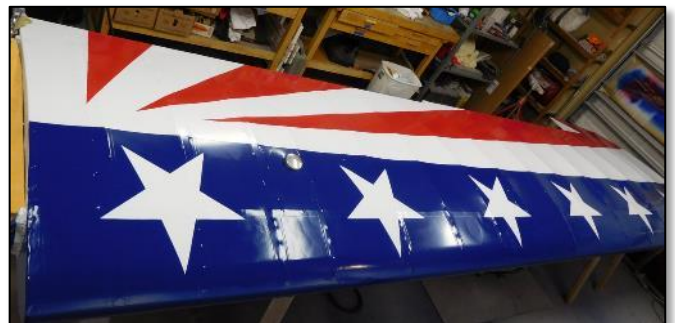
The flight controls and wings were sprayed with the white finish paint. Then the flight controls were temporarily attached to the wings in order to mask the
